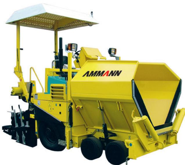
The machine has three axles: front, two axles for steering and rear, axle for traction. The rear axle is fitted with large pneumatic tyres so that the machine can be driven also on soft grounds. The actual version is equipped with four wheel drive traction as a standard. The steering system with a hydraulic pump gives a smooth control when turning. The hoppers are independently controlled by an electric-hydraulic system. The front
