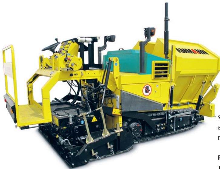
Tracked machine with rubber pads; automatic tensioning device system with grease accumulator. Hydrostatic transmission with two variable flow rate pumps which feed two motors with two displacements directly fastened to the planetary gearboxes which operate the tracks. Mounted on each pump, an electronic and proportional control gives a progressive start and stop, keeping the set speed constant. The steering-wheel is electronically controlled, the speed is constant when
