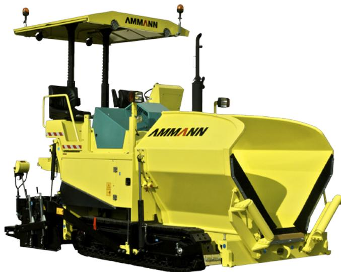
Tracked machine with rubber pads; automatic tensioning device system with grease accumulator. Hydrostatic transmission with two variable flow rate pumps which feed two motors with two displacements directly fastened to the planetary gearboxes which operate the tracks. Mounted on each pump, an electronic and proportional control gives a progressive start and stop, keeping the set speed constant. The steering-wheel is
